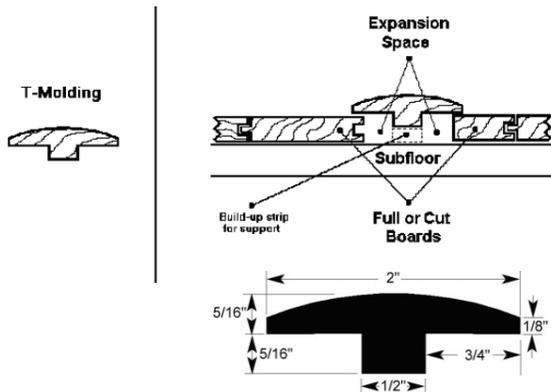
**T-Molding** - Covers the expansion space between two equal height flooring surfaces.
