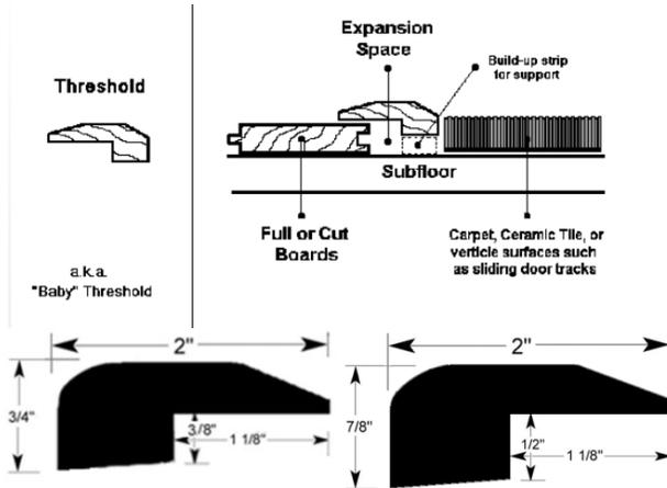
**Threshold** - Covers the expansion space at a threshold or sliding door.
