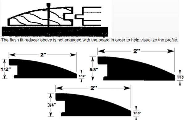
**Reducer** - Equalizes the level between two different height flooring surfaces.
